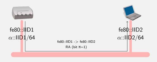
Router responds to RS with a RA message with bit  ${\tt M}$  set to 1. Host should request its IPv6 address from a DHCPv6 server.
