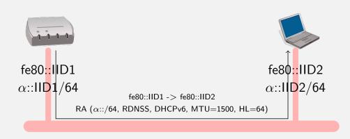
RFC 6106: IPv6 Router Advertisement Options for DNS Configuration proposes a new option for RA. It allows IPv6 routers to advertise a list of DNS recursive server addresses and a DNS Search List to IPv6 hosts.
