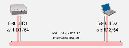
Host needs only static parameters (DNS, NTP,...). It sends an Information-Request message to All\_DHCP\_Agents multicast group. The scope of this address is link-local.
