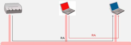
An attacker on the LAN can perform an attack by responding to RS messages
