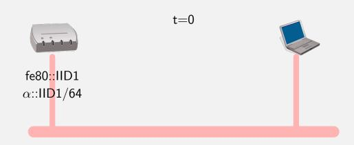
Time t=0: Router is configured with a link-local address and manually configured with a global address ( $\alpha$ ::/64 is given by the network administrator)
