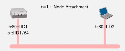
Host constructs its link-local address based on the interface MAC address
