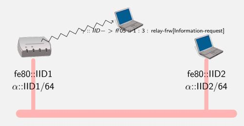
A relay (generally the router) encapsulates the request into a Forward message and sends it either to the All\_DHCP\_Servers site-local multicast group or to a list of pre-defined unicast addresses.
